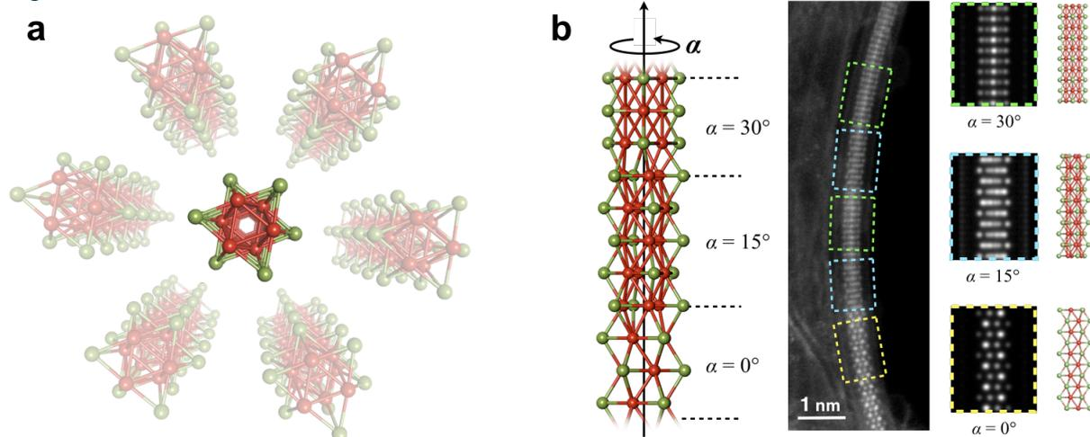
**Figure 1:** (a) A schematic image of transition metal monochalcogenide nanowire. (b) Torsional dynamics of a single MoTe nanowire confined within a CNT.
