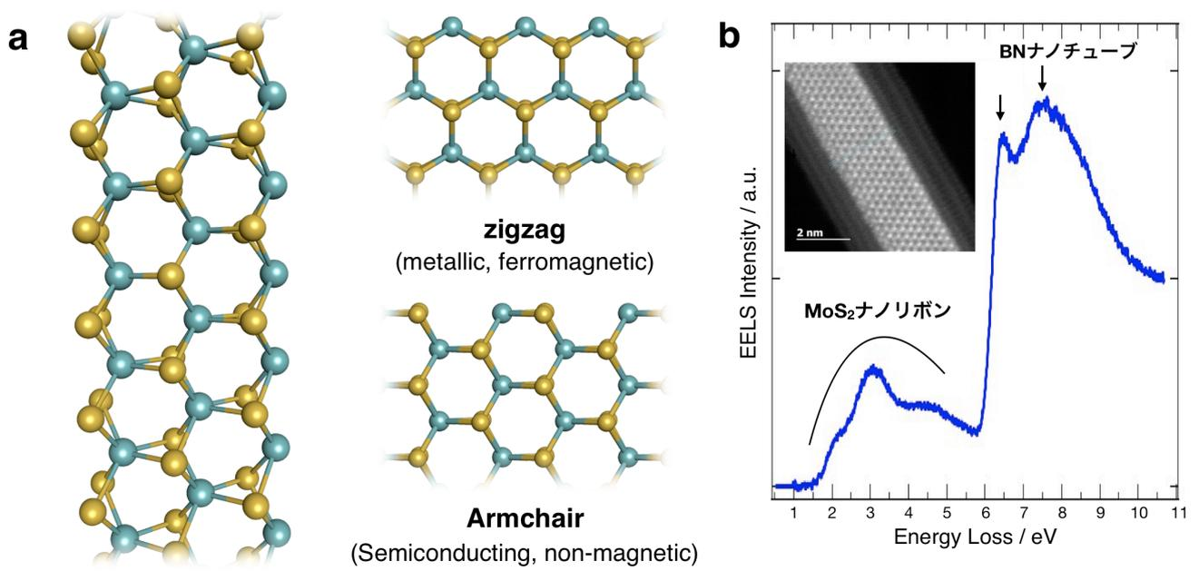
**Figure 2:** (a) A schematic image of transition metal dichalcogenide nanoribbon. (b) Atomic-resolution electron energy spectrum of an individual MoS<sub>2</sub> nanoribbons encapsulated inside a BNNT.
