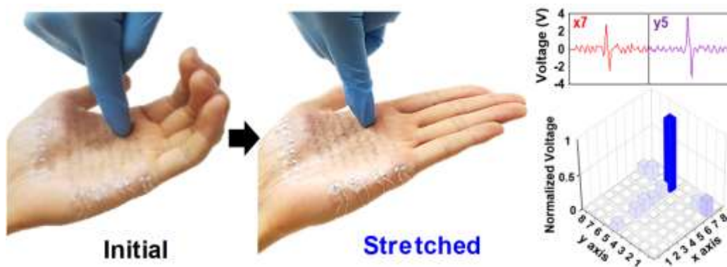
Figure 1: The optical image of stretchable/wearable self-powered touch sensor on the palm (left). The touch result at x7, y5 touch point of stretchable triboelectric touch sensor.
