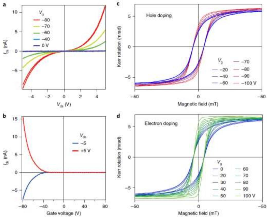
**Figure 1:** Kerr measurement of BN-encapsulated 3.5 nm  $\text{Cr}_2\text{Ge}_2\text{Te}_6$  sample with solid Si gate. a, I-V characteristics of the same device with five different fixed Si gate voltages measured at 40 K. b, Field-effect curves at 40 K with  $V_{\text{ds}} = -5$  and  $+5$  V (blue and red, respectively). c, d, Kerr angle measured at 40 K for negative (c) and positive (d) gate voltages respectively.
