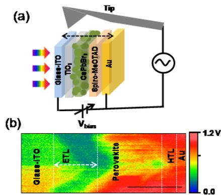
Figure 1: (a) Schematic diagram of the cross-sectional KPFM measurement system. (b) Surface potential image across the layers of the solar cell under solar illumination.
