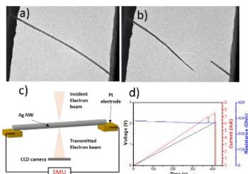
**Figure 1:** (a)-(b) TEM images of a Ag NW before and after failure due to Joule heating, (c) Schematic of the setup for in-situ TEM electrical characterization, (d) Voltage (current, resistance) vs. time curve.
