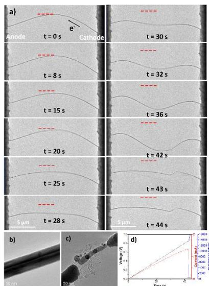
**Figure 2:** (a) Time-series of TEM images for the current-induced restructuring of a bent Ag NW (estimated bending strain of 0.21% and bending stress of 165 MPa) - the red dotted lines acts as a visual guide; (b)-(c) high magnification TEM images of the Ag NW in (a) before and after failure, respectively; (d) Voltage (current, resistance) vs. time curve.
